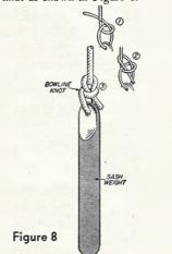
Replace the weight in the pocket and screw in place the section that was removed from the frame. Replace cord on the other side in the same manner. The sash can then be returned to its position in the frame and the moldings or bands holding it fastened.
