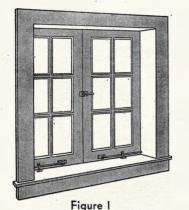
is one that is fastened to a frame with hinges and operates in much the same man-
