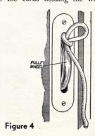
have to be removed from the sash. Loosen one cord at a time and tie a loop near the pulley as shown in Figure 4, so that it will not allow the weight to drop.
